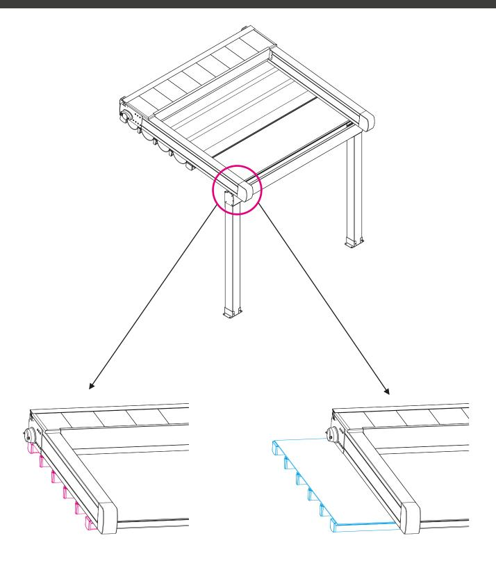
Counterweights can extend a minimum of 1cm from the rafter and a maximum of 80cm.
