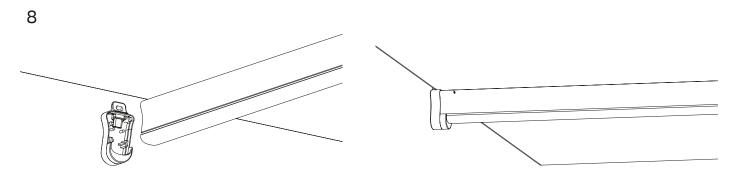
Finally, install all the plastic parts of the counterweights.
