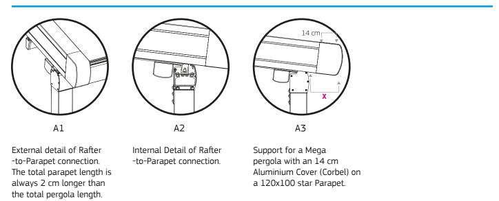
the **X** in images A3, A4 indicates the total overhang of the rafter from the parapet. The minimum overhang is equal to the aluminium cover. The recommended overhang is equal to the aluminium cover + 5 cm
