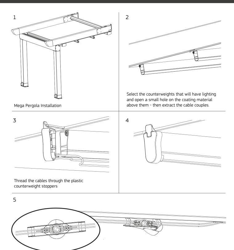
Connect the cables to the lighting fixture. Take one section of the cable found in the packaging and connect it from one lighting fixture to another
