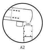
External detail of the Rafter -to-Parapet connection. The total parapet length is always 2 cm longer than the total pergola length. Mega pergola with a face rafter on the 160x120 parapet, 14 cm Aluminium Cover (Corbel).
