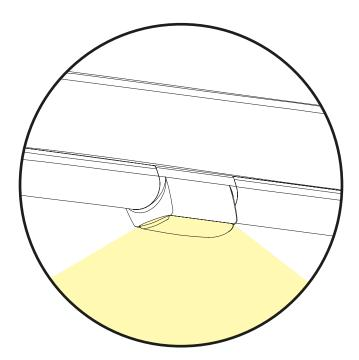
Lighting system with flat lighting fixtures. LED 12V lamps with a beam angle of up to 150°. In two lighting colours, Cool White and Warm White.
